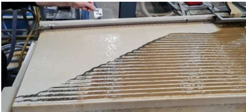
Figure 1: Beneficiation tests of W-tailings using a gravimetric Willey shaking table
