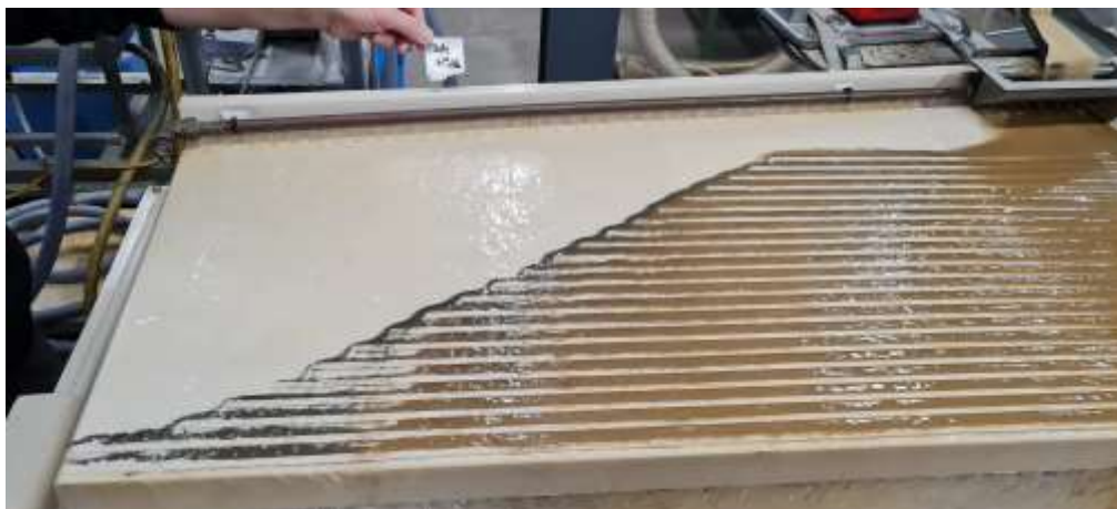
Figure 1: Beneficiation tests of W-tailings using a gravimetric Wilfley shaking table
