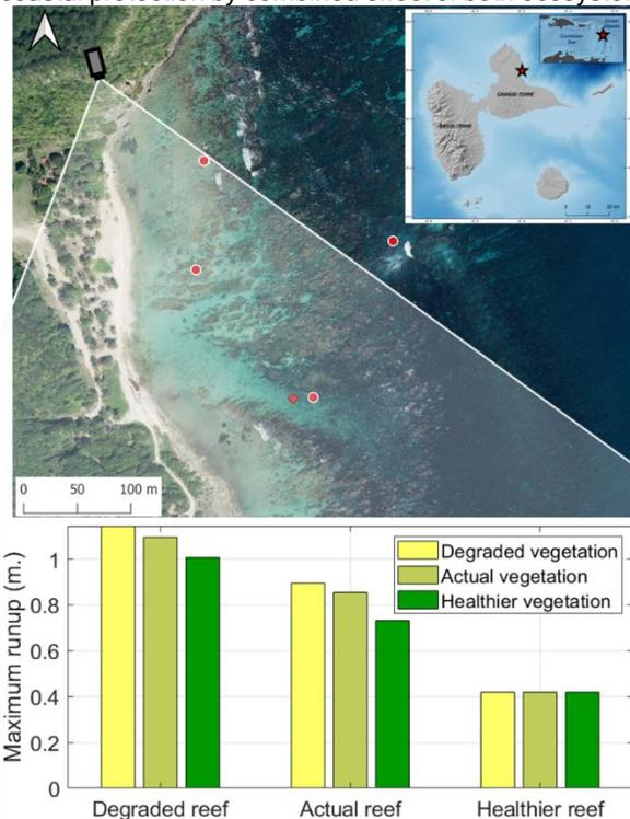
Figure 1 - Anse-Maurice beach map with sensors location (red markers), camera location (grey rectangles) and field of view (white area). Example of maximum runup for the same storm with different ecosystem states
