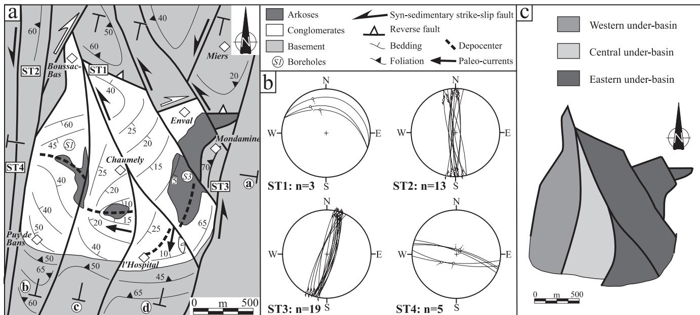
FIG. 6. – Structural data available on the Hospital coal basin and its borders. A. Structural map with bedding trajectories. Location of boreholes of figure 5, stereograms of figure 6b, and sections of figure 7. B. Microstructural data obtained on brittle fault zones that bound the basin. Lower hemisphere, equal area stereograms (see fig. 6a for location). C. Simplified map showing the relationships between the three under-basins and NNW-SSE to NNE-SSW-trending sinistral strike-slip faults.
