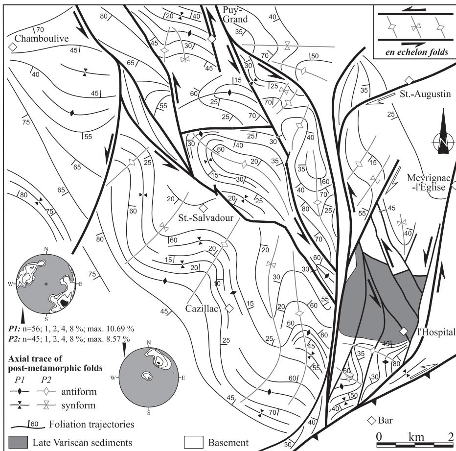
FIG. 4. – Map of  $S_{1-2}$  foliation trajectories and axial traces of two generations of post-metamorphic folds (see fig. 1a for location).
