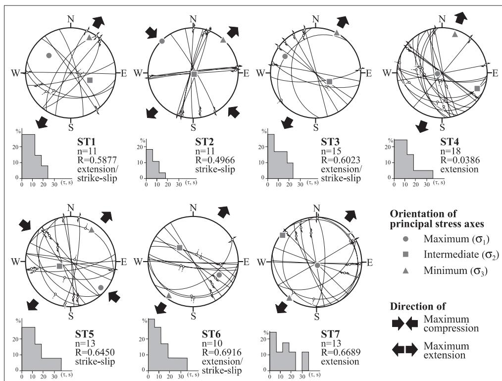
FIG. 2. – Fault-slip data and inversion obtained along the Argentat fault in the Hospital area. Stations are shown on figure 1a. Lower hemisphere, equal area stereograms. Histograms show the deviation between the striation (s) and the resolved shear stress ( $\tau$ ) for each fault plane. R is a stress ratio parameter defined as  $R = (\sigma_2 - \sigma_3)/(\sigma_1 - \sigma_3)$ .
