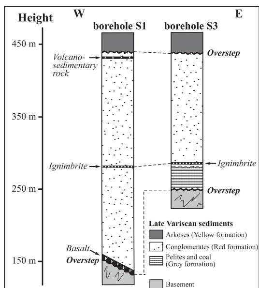
FIG. 5. – Synthetic boreholes through the Hospital basin [after Marest, 1985] (see fig. 6a for location).
