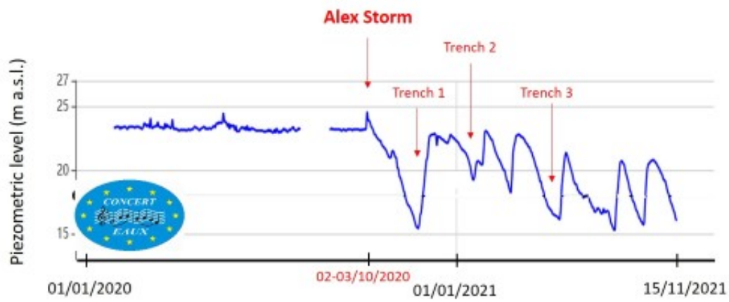
Evolution of the piezometric level at the Porra wellfield (Roya alluvial aquifer)
