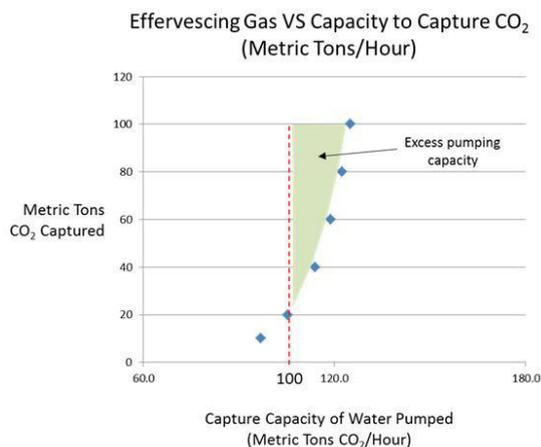
Figure 7 Effervescing gas versus capacity of the pumped water to capture CO<sub>2</sub>
