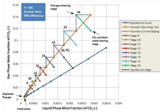
Figure 5 Modeled CO<sub>2</sub> absorption behavior in water using a multistage cascading absorber
