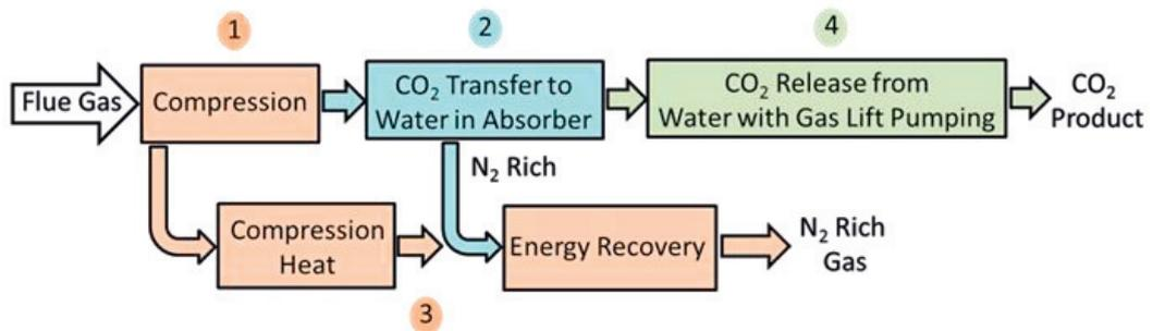
Figure 1 Generalized process steps for the Pi-CO<sub>2</sub> system
