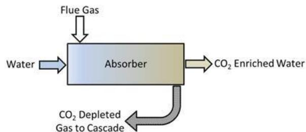
Figure 4 Simplified absorber diagram showing entries and exits
