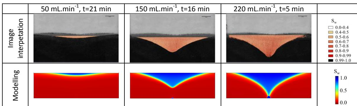
Figure 1: Comparison of measured (with image interpretation) and modelled cone of depression (0.5 mm GB) at the end of the pumping (steady-state condition) for different flowrates<sup>b</sup>
