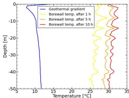
Figure 3. Natural geothermal gradient and temperature curves along the borewall after heat injection at 35°C during 1, 5 and 10 hours
