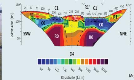
Resistivity tomography to identify the units geometry
