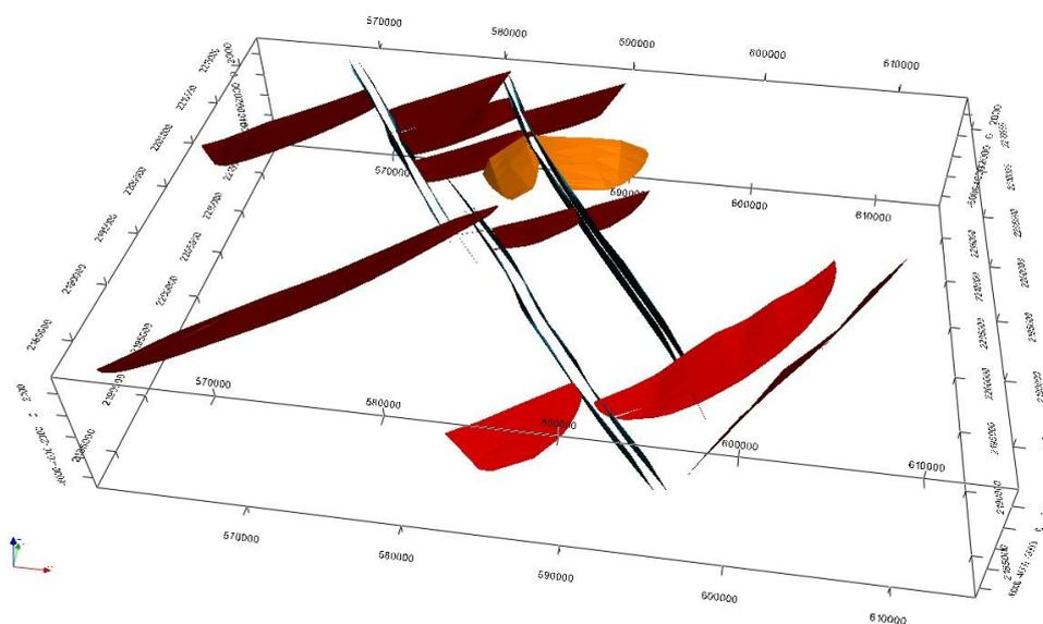
**Figure 10.** The 3D visualisation of the updated faults system including the ‘Damage zones’, modelled as delimited by two sets of NNW-SSE striking parallel faults. Coordinate system is WGS84/UTM zone 14N.
