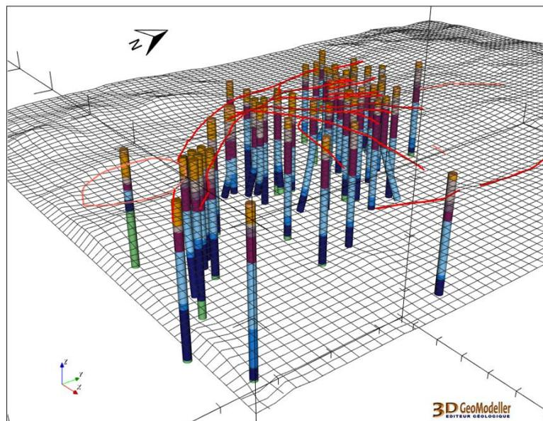
**Figure 6.** Fifty-six wells were used for the update of the Los Humeros local model. Ten of them are deviated. They are described according to the new geological description presented in Figure 5. DEM is displayed as a grid including the fault network traces (see Fig. 7).
