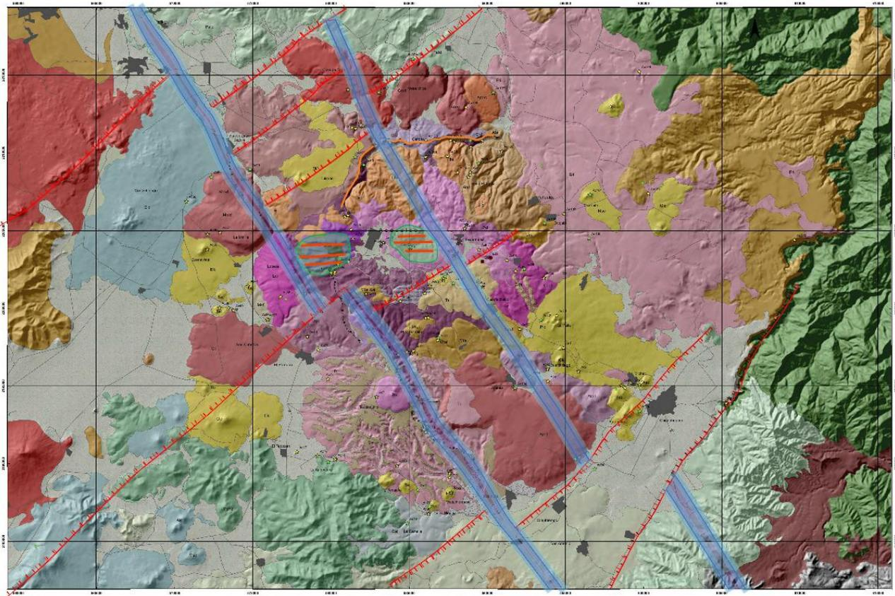
**Figure 9.** The updated geological map (modified after Avellan et al. 2019). The blue stripes represent the ‘damage’ zones, mainly including NNW-SSE striking fault segments. Differently, the SW-NE striking normal faults are indicated in red. In orange, the caldera fault traces. The two green with horizontal red lines showed two superficial alteration zones with a very shallow influencing.
