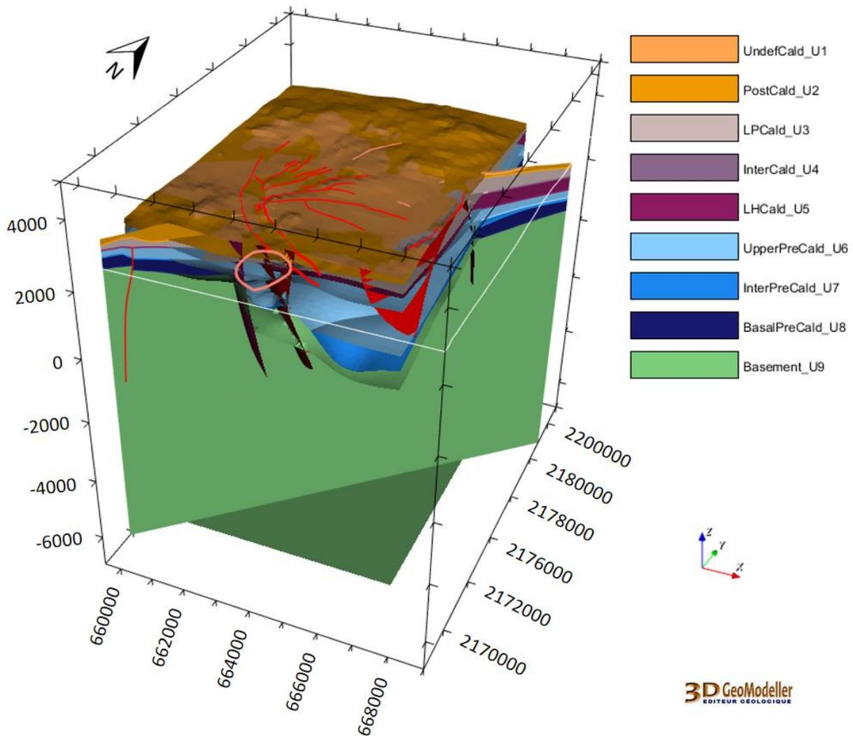
**Figure 8.** The 3D geomodel of Los Humeros updated at the local scale. It includes the updated faults (Fig. 7) and nine geological units listed on the right hand side (see also Fig. 5). Coordinate system is WGS84/UTM zone 14N.
