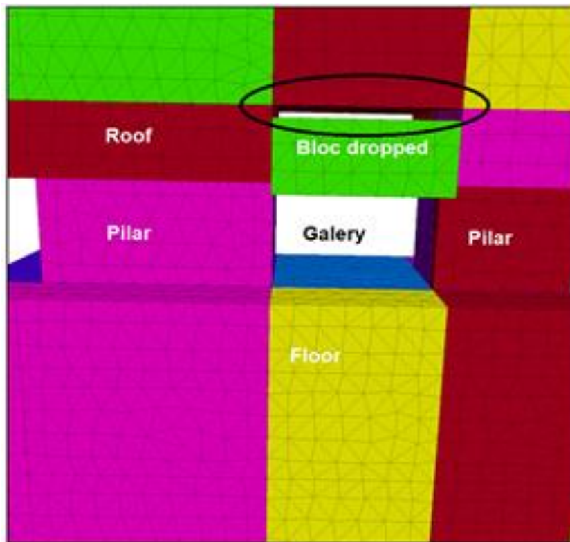
Figure 7. Simulation of the vault collapse induced by a decrease of cohesion and friction parameters.
