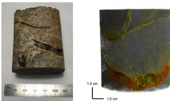
**Figure 3 : Three-dimensional observations of samples comes from "Peyrouse 1 borehole". Red color corresponds to mineralization (lead sulphides). The yellow colour correspond to the planar porosity located on the fracture walls (resolution of the figure is 25 µm).**
