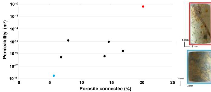
**Figure 5 : Connected porosity and permeability measurements (according to the Heap & Kennedy (2016) method). In blue, sample 4-4-1 has a low degree of alteration. In red the sample 19-1-1 with a high degree of alteration. These purely qualitative degrees of alteration are based on macroscopic, microscopic observations and three-dimensional visualization by X-ray microtomography analysis.**
