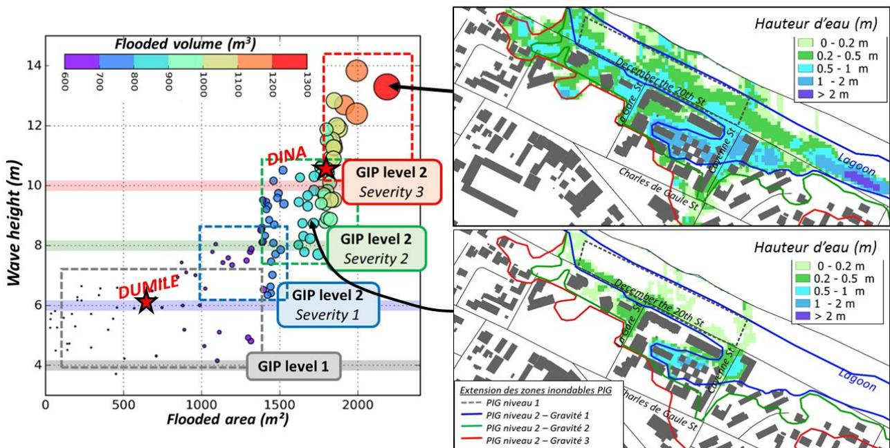
**Figure 5:** Right panel: Relationship between maximum coastal wave heights (at 50m-depth) with maximum flooded areas and overtopping volumes in the city centre of Sainte Suzanne. Left panel: Two examples of flood maps compared with the GIP contours.
