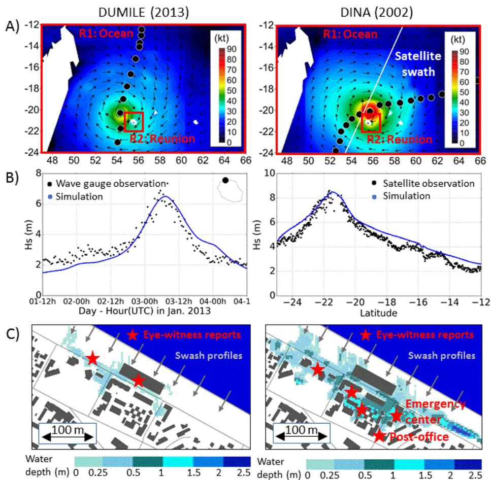
**Figure 2:** A) Grid extent with tracks (black dots), wind intensity (colors) and directions (arrows) of cyclones Dina and Dumile calculated with MESO-NH from best-track data. B) Comparison between simulated wave heights with observations from satellite altimetry on January the 23<sup>rd</sup> at 06 UTC (Dina) or time-varying observations from buoy RN4 (Dumile). C) Position of the SWASH profiles and comparison between simulated flooding with eyewitness accounts.
