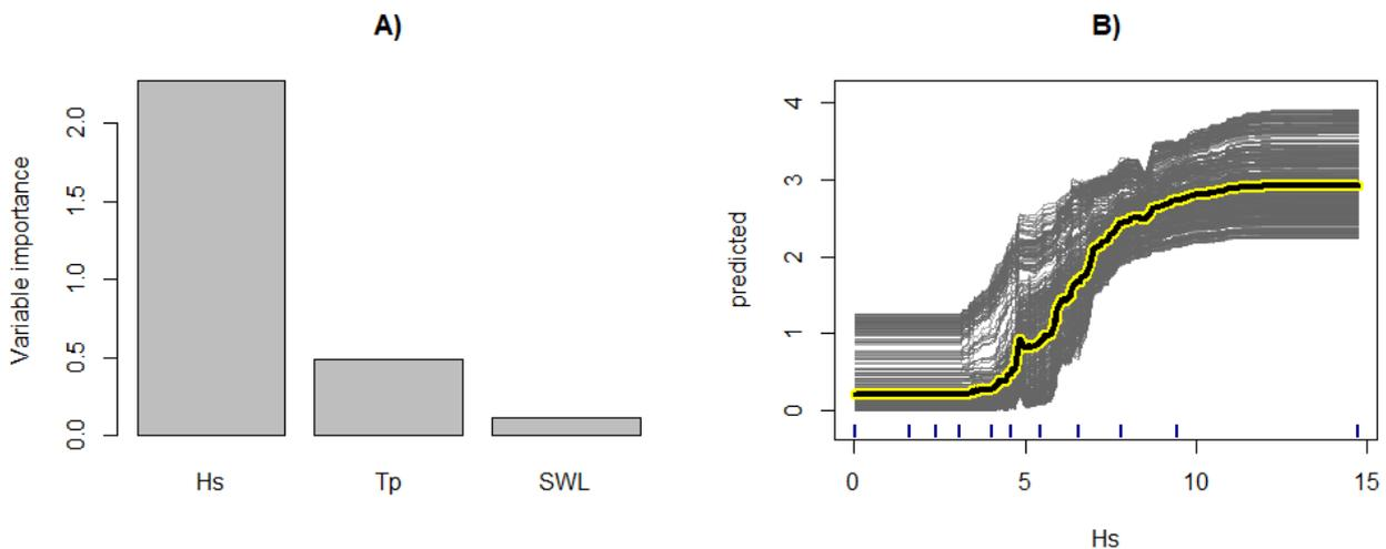
**Figure 4:** A) Importance measure for each variable ( $H_s$ ,  $T_p$ ,  $SWL$ ) derived from a random-forest model trained using the synthetic cyclones B) Functional relationship between the predicted value of the log-transformed of  $V$  and  $H_s$ . The yellow line indicates the average effect of  $H_s$ .
