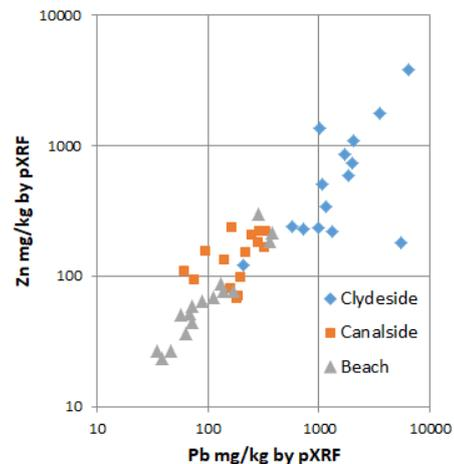
**Fig. 1:** Pb and Zn concentrations by pXRF (mg/kg) in soil and Clyde beach sediment.
