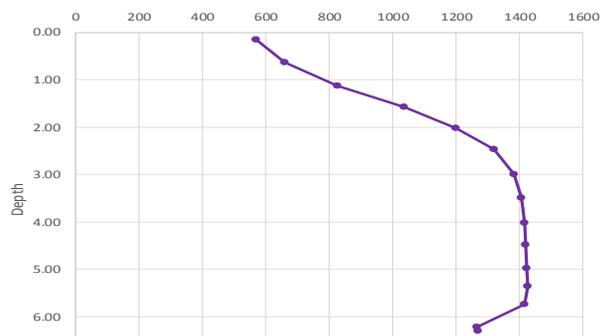
**Fig. 2:** Conductivity profile by multiparametric probe ( $\mu$ S/cm) in shallow groundwater, BH19.
