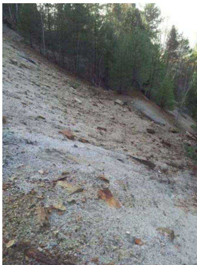
Figure 8: As-bearing coarse gravity sorting residues in dumps
