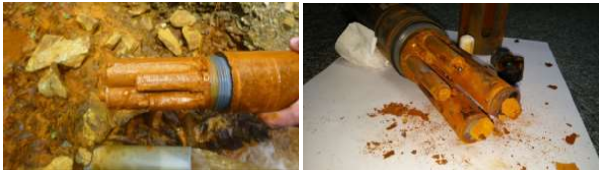
Figure 6 : The probe as recovered (left) and after gentle wiping (right)
