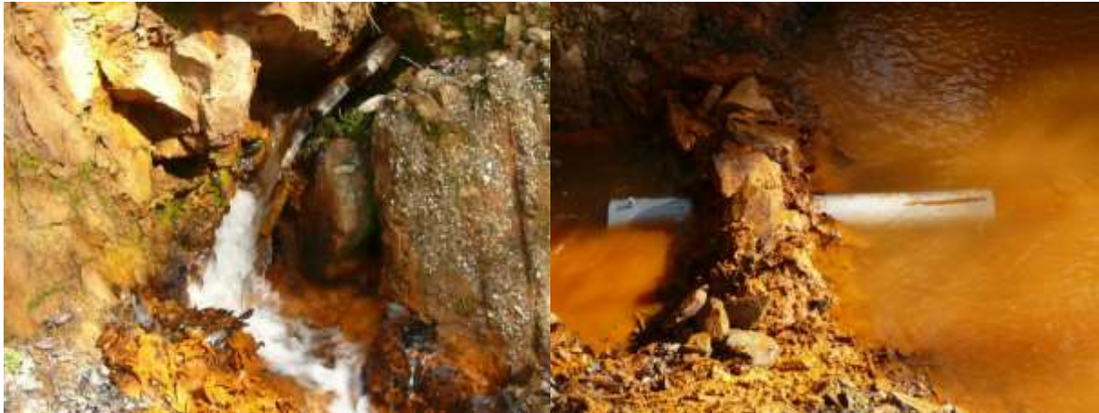
Figure 5 : Mine drainage spring (left) and pipe hosting the multiparametric probe (right)
