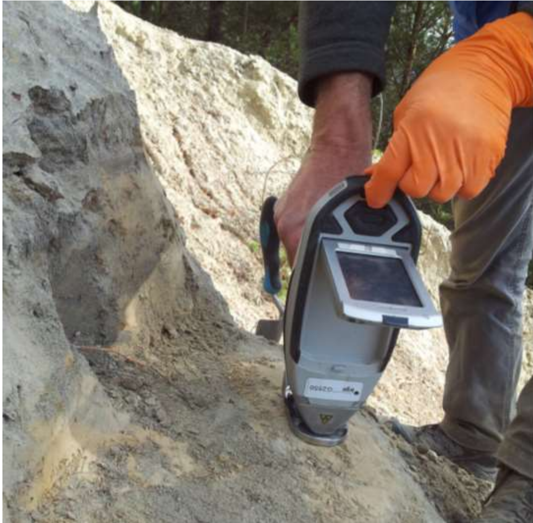
Figure 4: On-site analysis of residues using pXRF
