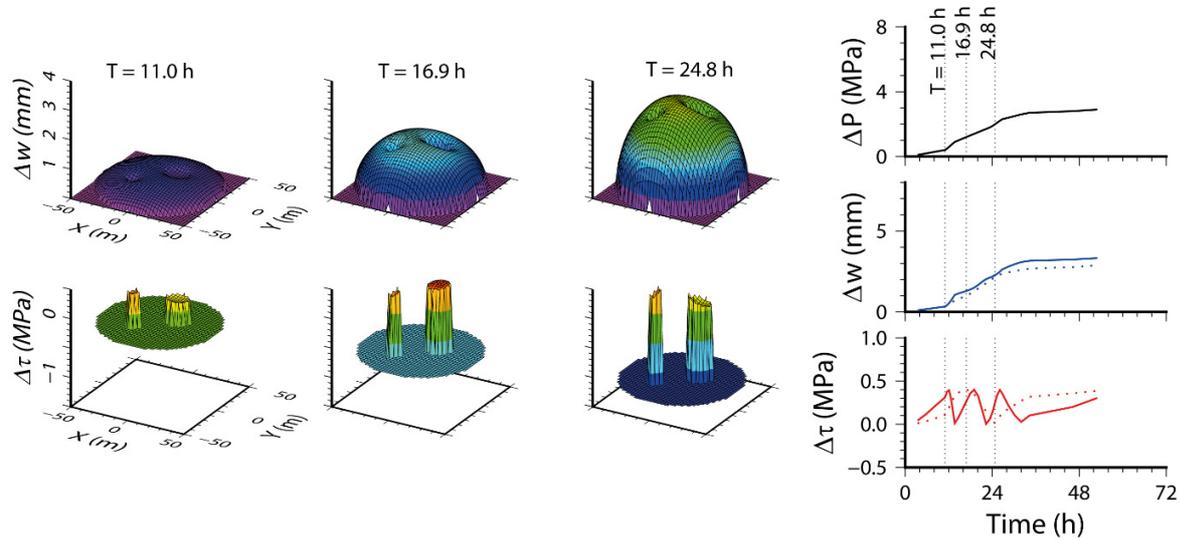
Figure 2. Snapshots of fault slip and shear stress change on the fault segment at three different times. Pore pressure change ( $\Delta P$ ), fault slip ( $\Delta w$ ) and shear stress change ( $\Delta \tau$ ) are shown on the right. Schematic illustration of TOUGH2-BIEM simulations of fluid driven faulting process. (left). Solid and broken lines correspond to small and large asperities of radius 5 m and 10 m, respectively.
