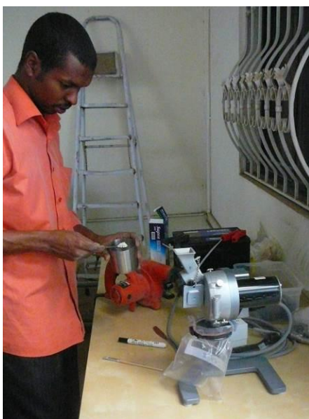
Figure 3: On-site battery operated sample milling device
