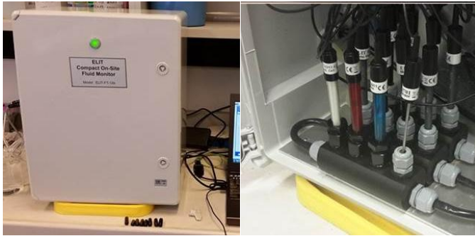
Figure 10: Fluid Management System consisting of a peristaltic pump and 12 ion selective electrodes (photo Nathan Reid, CSIRO)
