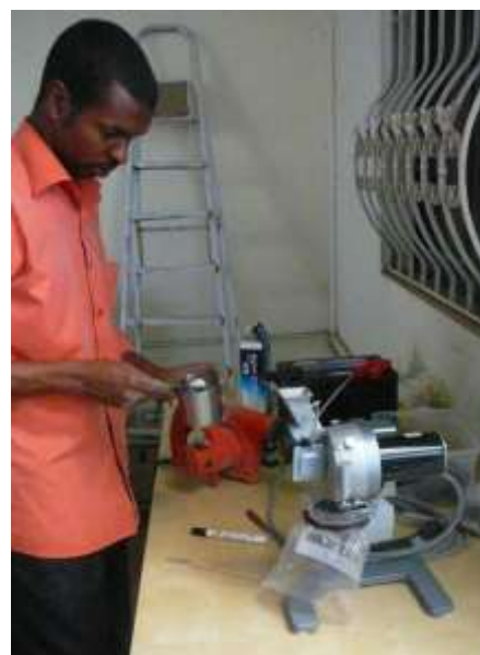
Figure 3: On-site battery operated sample milling device
