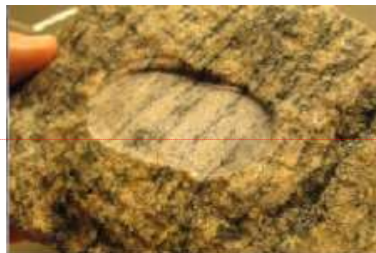
Figure 2: Abrasion surface for pXRF measurements (photo K. Esbensen)
