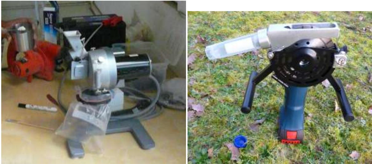
**Fig. 4** Sample preparation equipment running on batteries
