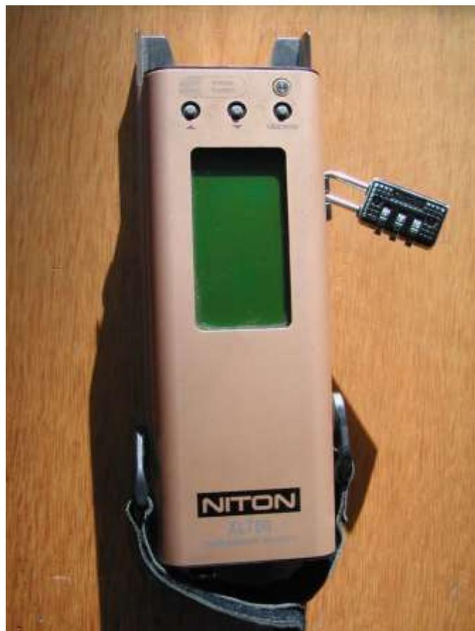
*Fig. 1 An early radioactive source pXRF spectrometer*
