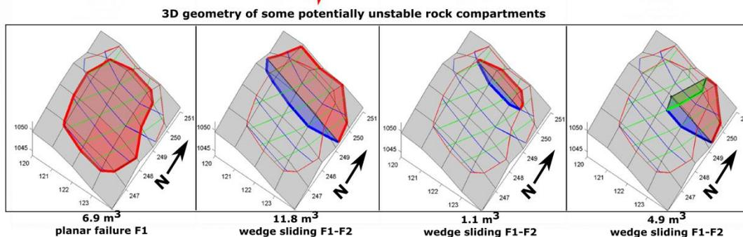
**Figure 1: Result of block partitioning of a 1-m resolution DEM in Corsica based on three fracture sets recognized by field investigations. Considering that each fracture set has a 1-m-period, this figure illustrates how rock blocks could fail by planar sliding on single family fracture or by wedge rupture rooted on different pairs of fracture planes.**
