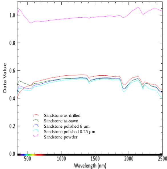
Figure 2: Spectra of Sandstone – Intensity of the reflectance.
