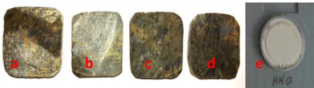
Figure 7: Peridotite samples – a: as-drilled; b: as-sawn; c: polished at 6 μm; d: polished at 0.25 μm; e: crushed to powder.
