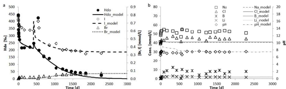
**Figure 1. Comparison of experimental data measured over the time in the MVE long term test to the modeling results obtain with the GRAAL model and Phreeqc; a. deuterium, iodine and bromide; b. sodium, chlorine, boron, lithium and pH.**
