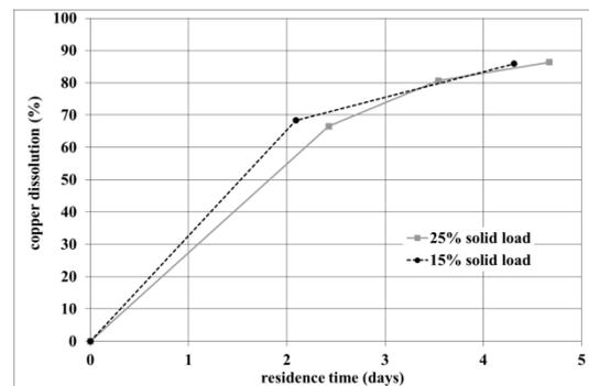
Figure 2. Influence of solid load on copper dissolution
