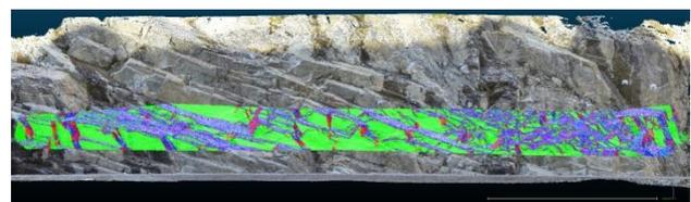
Figure 2. 3D RGB point cloud with a 1m-high area of interest around the scan line survey where normal are colored by HSV.
