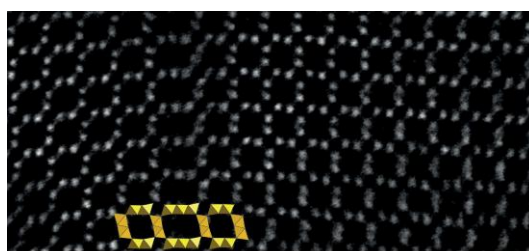
Figure 1. STEM observation of cryptomelane formed from vernadite precursor [2]. Bright spots are individual Mn atoms. Overlaid yellow octahedra at the bottom left of the image materialize MnO 6 octahedra.
