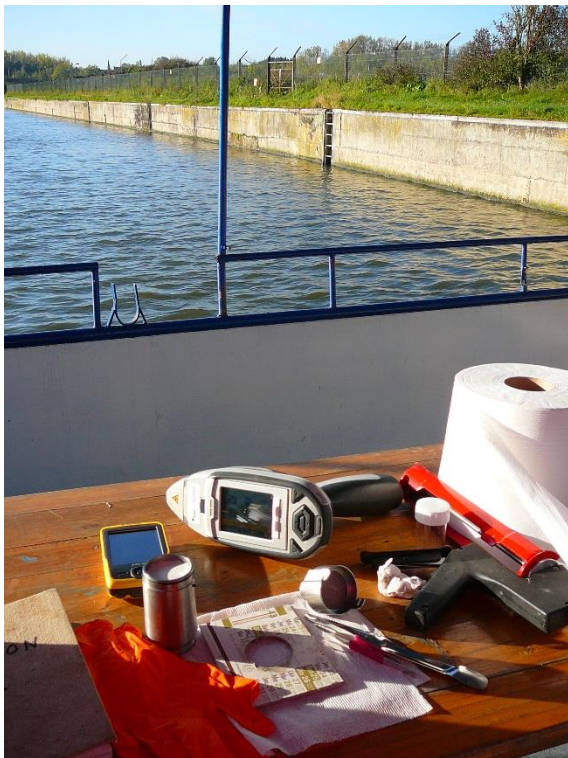
Fig. 2 pXRF analysis onboard a sampling boat.
