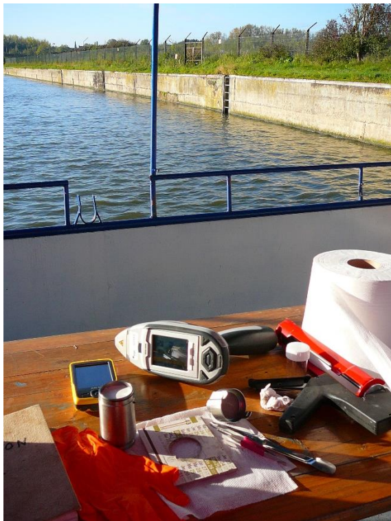
Fig. 2 pXRF analysis onboard a sampling boat.
