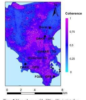
**Figure 7.** Mean coherence of the ERS and Envisat interferograms selected to compute ground motion velocity trends over 1993–2010. White contour lines are plotted for the following coherence values: 0.25; 0.5; 0.75.
