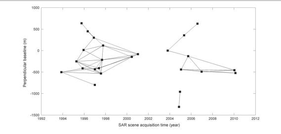
**Figure 3.** Baseline/time diagram for the ERS1, ERS2 and ENVISAT data. This diagram displays the selected SAR scenes (squares) and interferograms (segments) used to compute the following ground motion velocity maps. These scenes and interferograms meet the requirements in terms of baseline, time span, coherence and limited atmospheric effects. The ordinate axis origin is set to zero for the master scene of both Envisat and ERS stacks of interferograms (SAR scene acquired on 23rd October 2003).
