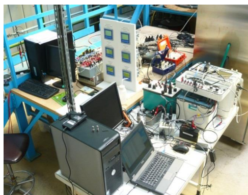
Figure 2. Setup up and apparatuses for the monitoring of the physical and chemical parameters of the column output water and geophysical electrical measurements into the column (and over the length of the column)
