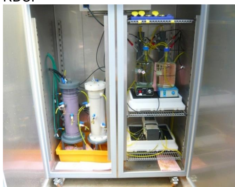
Figure 1. Complete experimental device of percolation (feed bottles with reagents and pollutants, pumps, columns, flow-through-system carrying the monitoring probes), placed in air-conditioned cupboard
