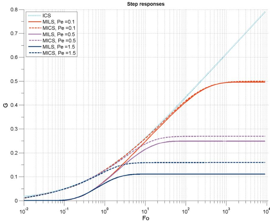
**Figure 4: Computed step responses for  $Pe = 0.1, 0.5, 1.5$  as a function of the Fourier number  $Fo$  (normalized time). ICS: infinite cylindrical source; MILS: moving infinite line source; MICS: moving infinite cylindrical source (new approach).**
