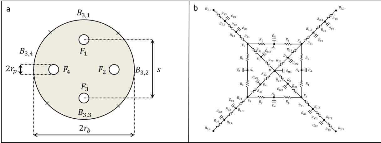
**Figure 5: (a) cross-sectional view of the PHE geometry. (b) The developed RC model.**
