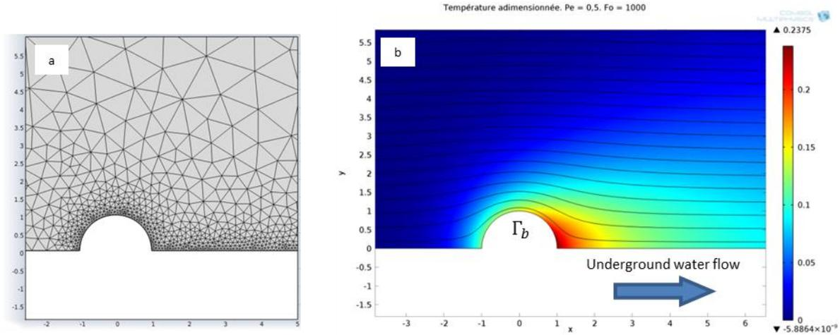
**Figure 3: (a) Domain mesh. (b) Computed normalized temperature  $T^*$  and streamlines in the borehole surrounding at normalized time (Fourier number)  $Fo = 1000$ . In this simulation the Peclet number  $Pe$  was set to 0.5. The water flows rightwards.**
