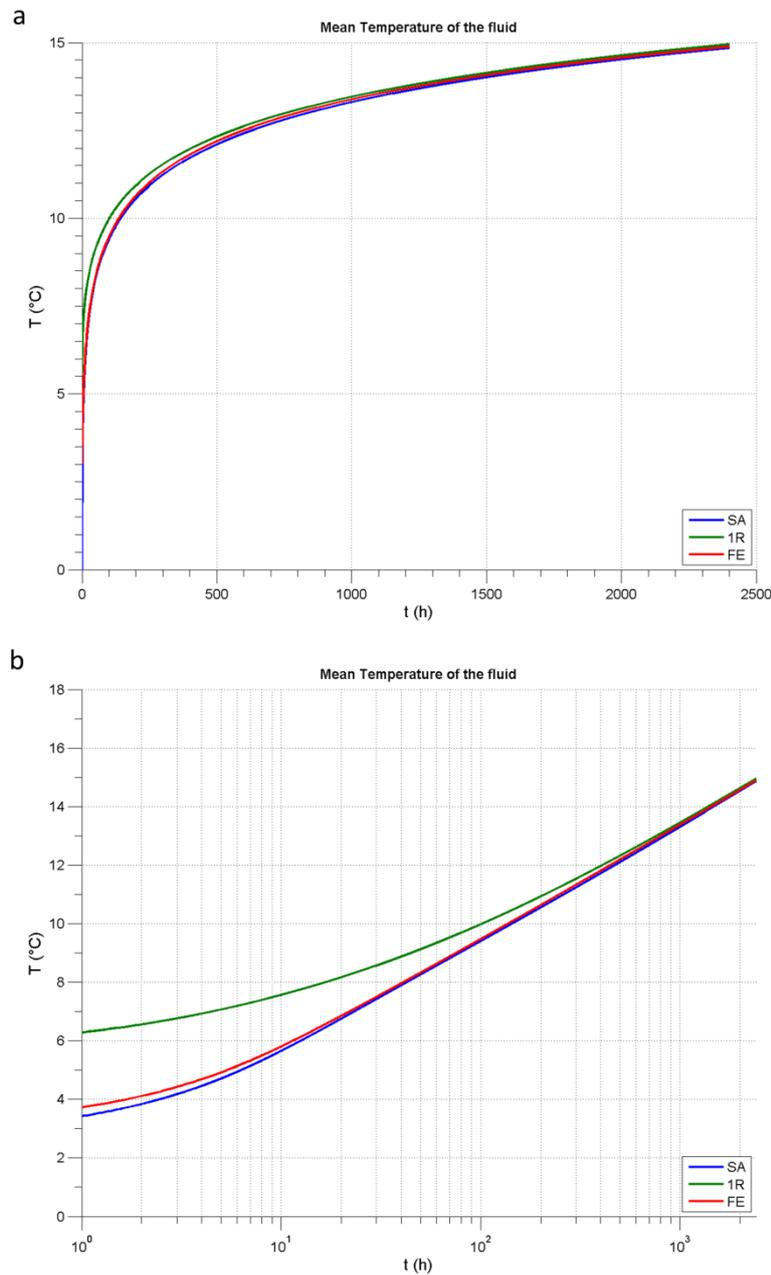
**Figure 7: Evolution of mean temperature fluid  $T_{fl}$  computed by the three models in normal scale (a) and in semi-logarithmic scale (b).**
