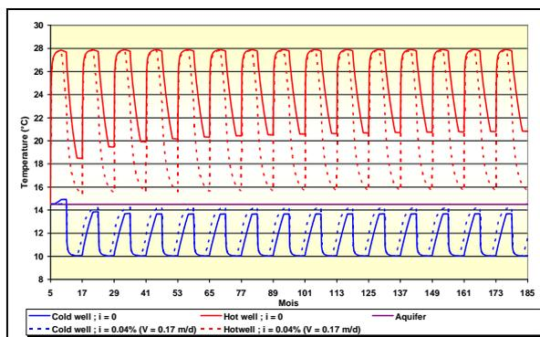
Figure 5: Comparison of the simulated temperatures in the cold and hot wells for  $i = 0$  ( $V = 0$ ), and  $i = 0.4\text{‰}$  ( $V = 0.17$  m/d) ;  $Q = 50$  m<sup>3</sup>/h, Aquifer thickness = 25m, Cover thickness = 20m,  $K = 5.10^{-3}$  m/s,  $\varepsilon = 15\%$ .
