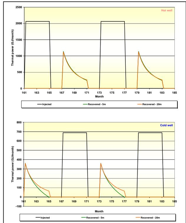
**Figure 9:** Comparison of simulated “useful” thermal power in the cold and hot wells for cover thickness 5 and 20m ; other parameters same as in Figure 8.
