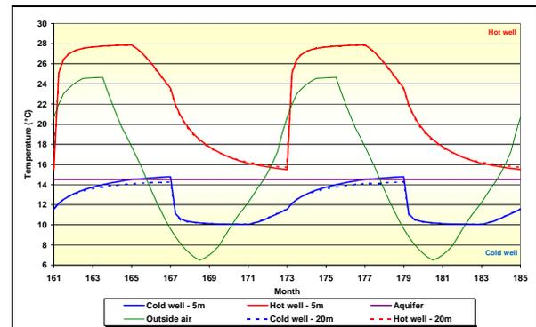
**Figure 8:** Comparison of the simulated temperatures in the cold and hot wells for cover thickness 5 and 20m ;  $Q = 50$  m<sup>3</sup>/h,  $L = 200$ m, Aquifer thickness = 25m, Cover thickness = 20m,  $K = 5.10^{-3}$  m/s,  $\epsilon = 15\%$ ,  $i = 0.4\%$ .
