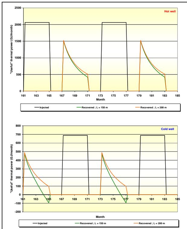
Figure 11: Comparison of simulated “useful” thermal power in the cold and hot wells for L = 150 and 200m ; other parameters same as in Figure 10.
