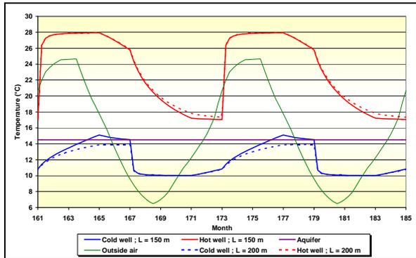
Figure 10: Comparison of the simulated temperatures in the cold and hot wells for L = 150m and 200m, i = 0.4‰; Q = 50 m<sup>3</sup>/h, Aquifer thickness = 10m, Cover thickness = 20m, K = 5.10<sup>-3</sup> m/s, ε = 15%.
