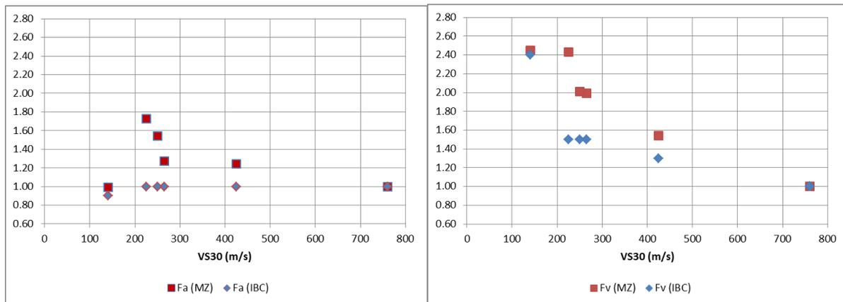
Figure 10. Comparisons of amplification factors Fa (left) and Fv (right) found for this microzonation (MZ) and proposed in IBC code.
