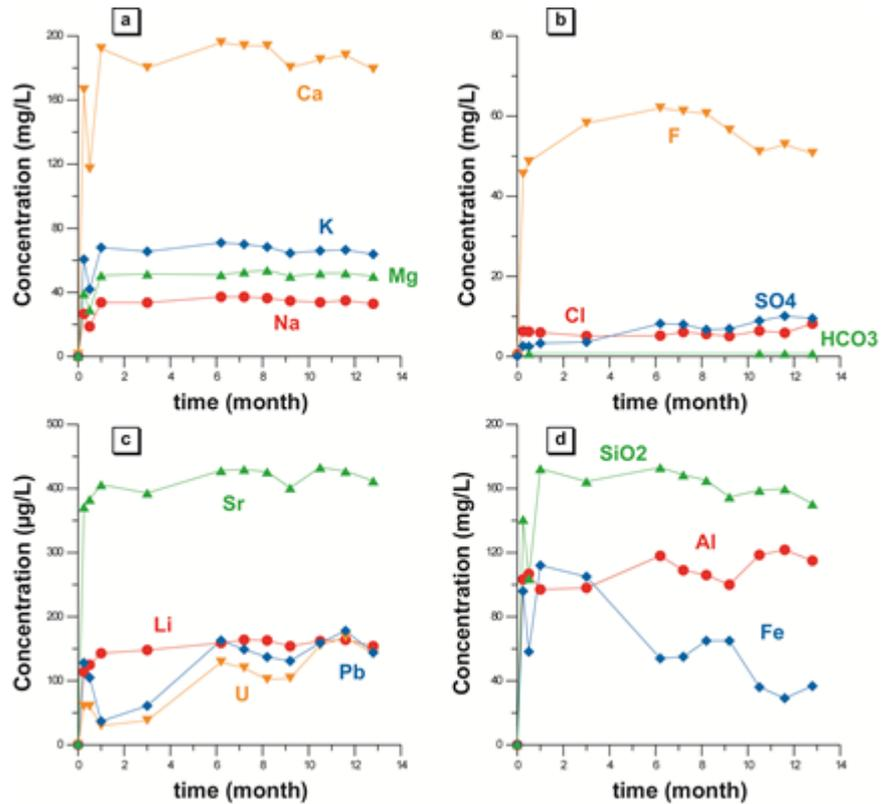
Fig. 1. Graphs showing the evolution over time of (a) cations concentrations (Na, K, Mg and Ca in mg/L); (b) anions concentrations (Cl, SO<sub>4</sub>, HCO<sub>3</sub> and F in mg/L); (c) trace elements concentrations (Li, Pb, Sr and U in µg/L); (d) SiO<sub>2</sub>, Al and Fe concentrations in mg/L.
