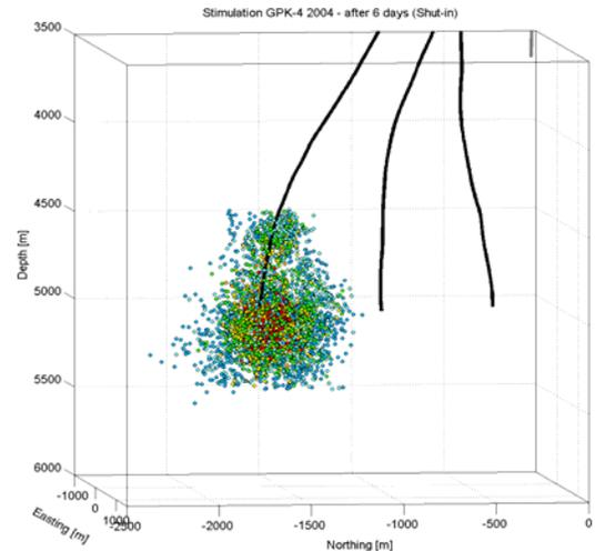
Figure 8: Microseismic locations of GPK4 in 2004
