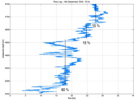
Figure 7: Flow log during stimulation of GPK4
