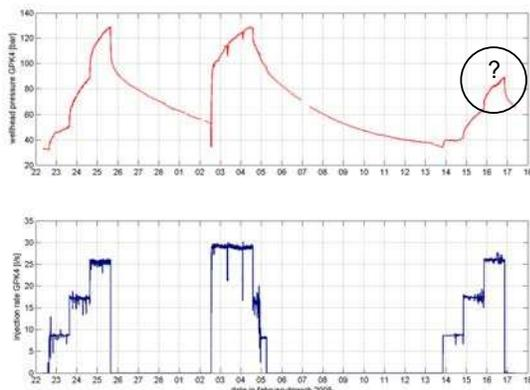
Figure 11: Pressure and flow for the acidization test
