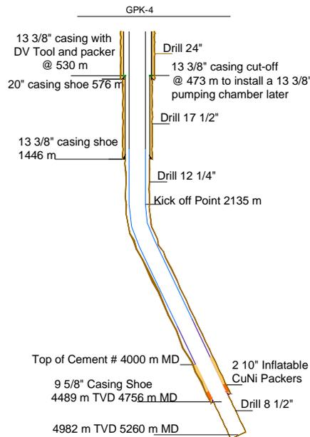
Figure 5: Completion of highly deviated well GPK4
