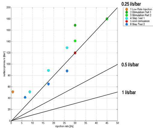
Figure 13. Plot of injected pressures & flow in GPK4
