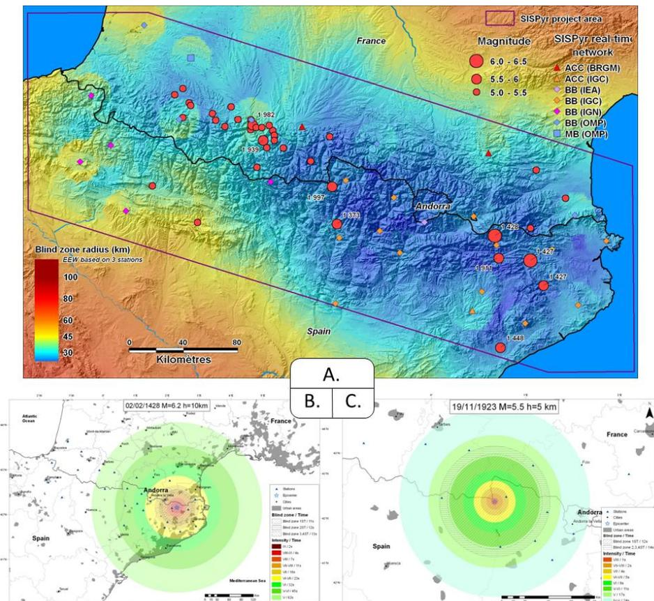
**Figure 1.** Simulated performances of a virtual Pyrenean EEW based on the SISPy network A. Extension of the blind zone in function of the epicentre location with an EEW using a minimum of 3 stations. SISPy seismic real-time network is also represented as well as the historical Pyrenean seismicity. B. and C. Intensity attenuation versus extension of the blind zone for scenario earthquakes corresponding respectively to the M6.5-1428 & M5.6-1923 damaging events.
