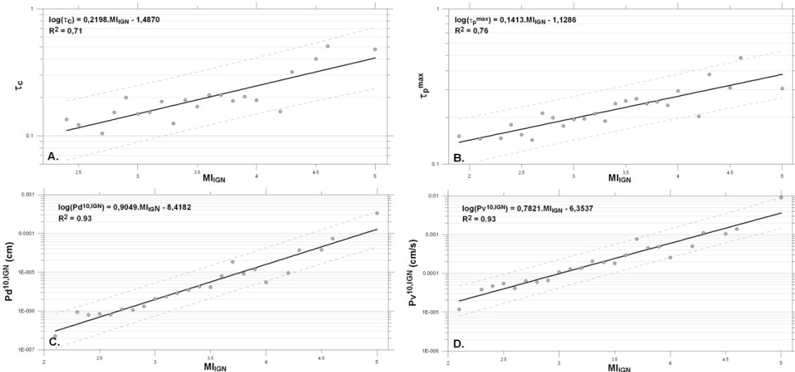
**Figure 4** A, B, C and D. Empirical correlations linking proxy parameters  $\tau_c$ ,  $\tau_p^{\max}$ ,  $P_d^{10}$  and  $P_v^{10}$  (mean per event) with IGN local magnitude for Pyrenean earthquakes. Calculations carried out on the traces of the catalogue that satisfy the selection criteria (analysis interval set at 3 s). The straight line obtained by linear regression is shown in black, while the grey dashed lines indicate the confidence interval at 95 % for a new observation.
