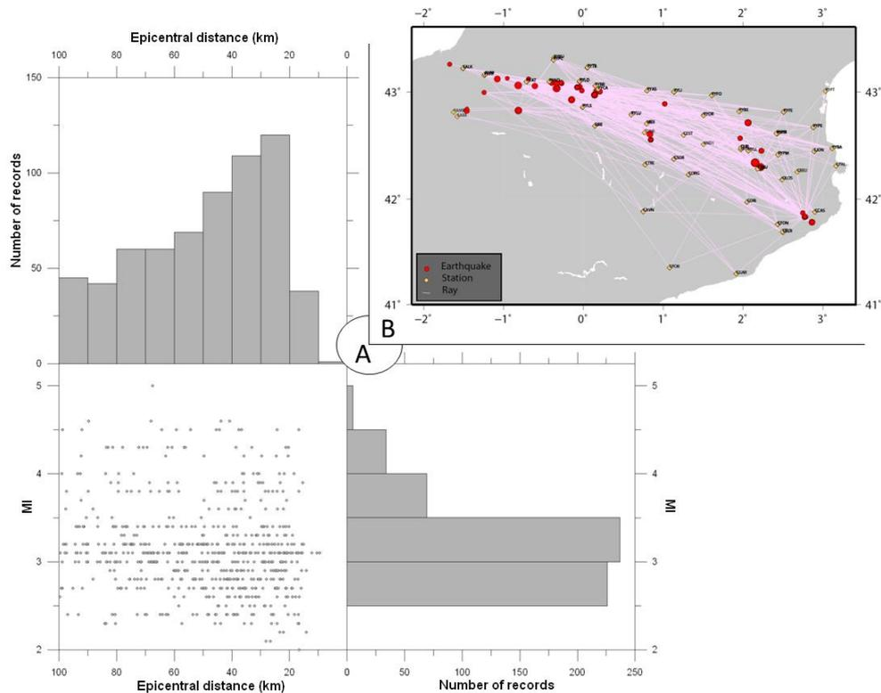
**Figure 3.** Representation of the study data-set. A. Distribution of the seismic signals versus magnitude and epicentral distance. B. Map of earthquakes included in the catalogue and of corresponding recording seismological stations.
