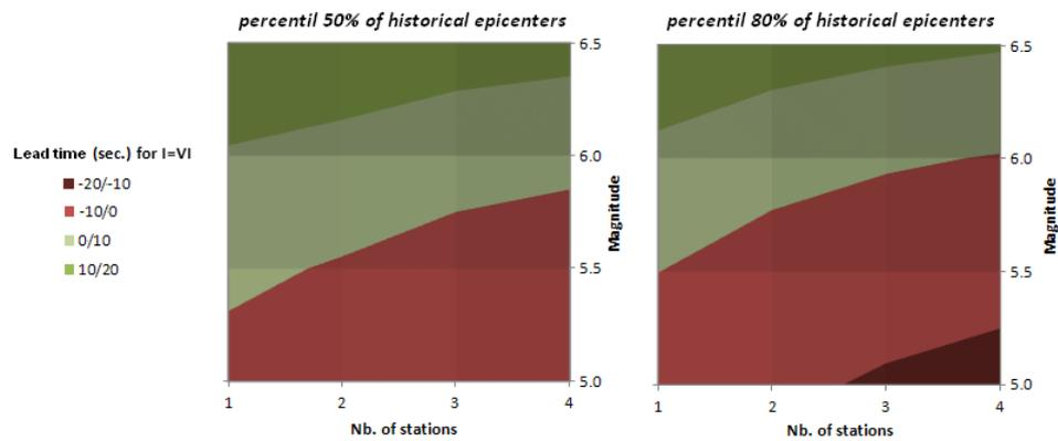
**Figure 2.** Simulated performance at regional scale of a Pyrenean EEW confronting past seismicity to estimated blind zones' extension. Configurations for which 50% (left) and 80% (right) of historical epicentres lead to positive lead times (i.e. blind zones smaller than isoseist  $I=VI$ ) are indicated thanks to green colour gradation, while negative values are indicated thanks to red colour gradation.
