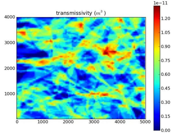
Figure 21: Productive layer transmissivity ( $\text{m}^3$ )
