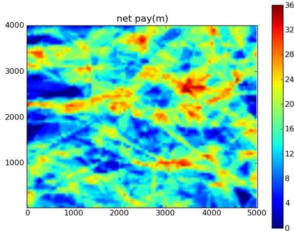
Figure 20: Productive thickness in the homogeneous model ( $K_h \geq K_{min} = 5.10^{-14} \text{ m}^2$ )
