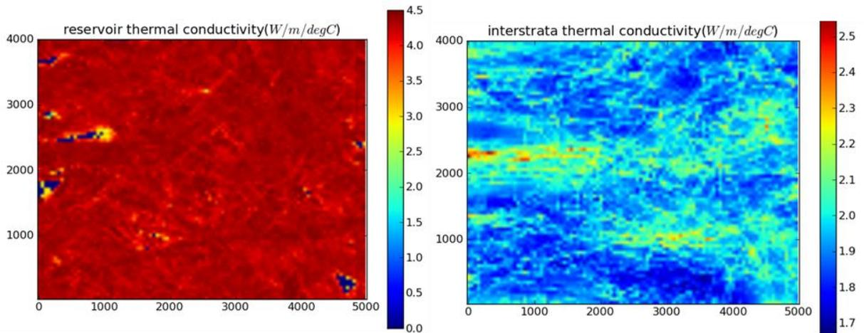
Figure 24: Reservoir and interstrata thermal conductivity (W/m/°C)
