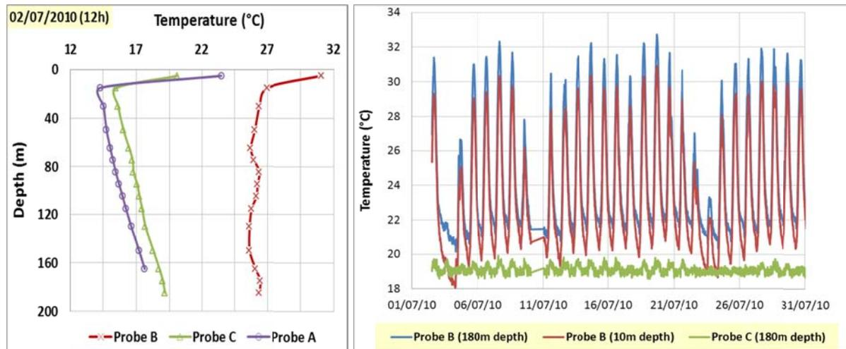
Figure 1: Temperature vertical distribution and temporal evolution in the schist rock after 3 months of solar thermal energy injection
