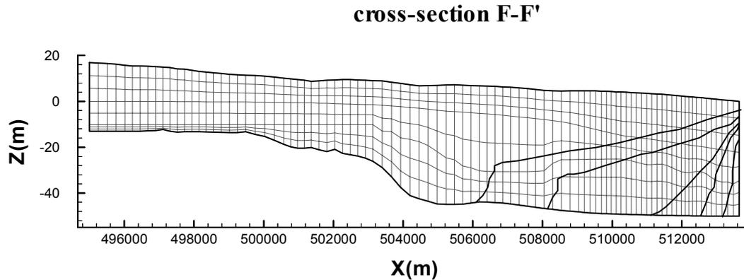
Figure 5. Cross-sectional view of the seawater intrusion; simulated moving interface positions from 1974 to 2006 with 8 years interval are plotted.
