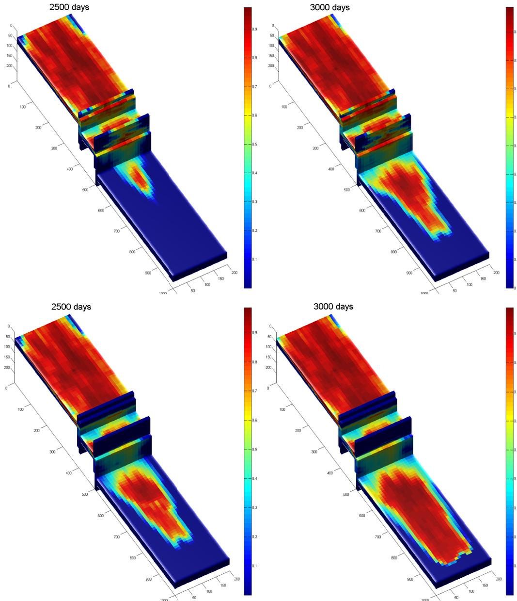
Figure 2: CO<sub>2</sub> saturation maps after 2500 and 3000 days of injection for case 1 (top) and case 2 (bottom).
