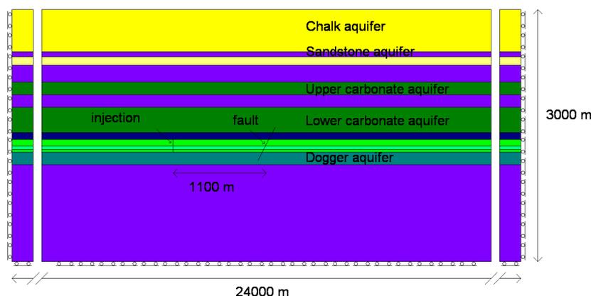
Figure 1: Schematic view of the Paris basin model
