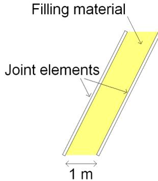
Figure 2: Schematic view of the fault model
