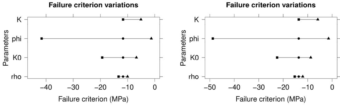
Figure 5: Comparison of parameters effect on the Mohr-Coulomb failure criterion
