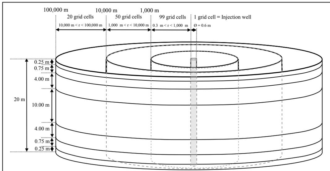
Figure 2: Geometrical 2D radial model for supercritical CO<sub>2</sub> injection in a carbonate reservoir. The diameter of the injection well is 0.6 m whereas the first element adjacent to the wellbore presents a width of 0.32 m.
