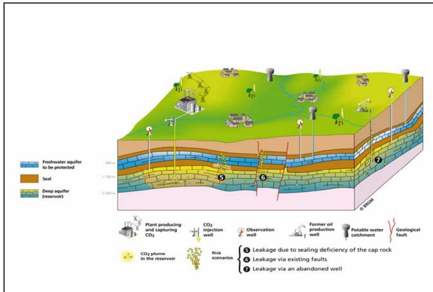
Figure 1: Potential leakage pathways from a CO<sub>2</sub> storage reservoir (adapted from Bouc et al., 2009)
