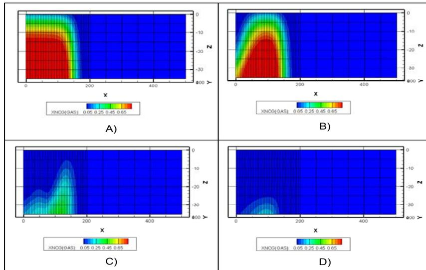
Figure 3 : CO<sub>2</sub> mass fraction in the vadose after 6 months of operation for four remediation strategies: A) natural attenuation; B) extraction through a single vertical well; C) extraction through three vertical wells and D) extraction through one vertical well and two horizontal conduits.
