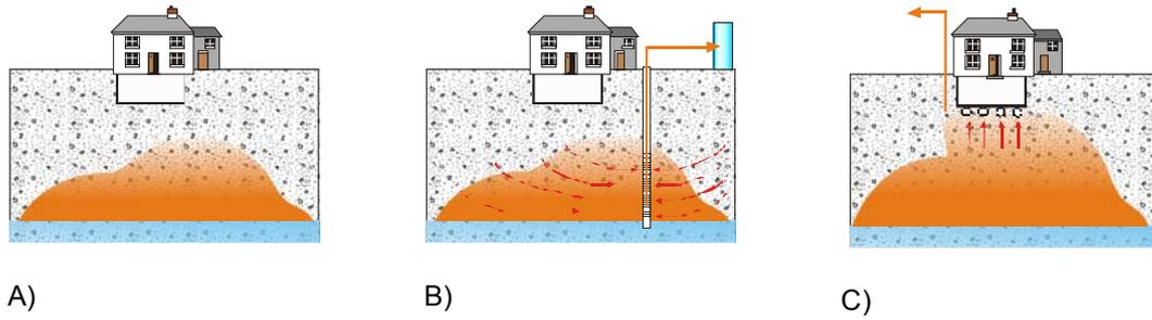
Figure 2: intervention strategy for managing the transfer of CO<sub>2</sub> within the vadose zone : A) monitored natural attenuation ; B) active extraction techniques such as SVE; C) protection of targets through techniques aiming at stopping the vertical migration of CO<sub>2</sub>
