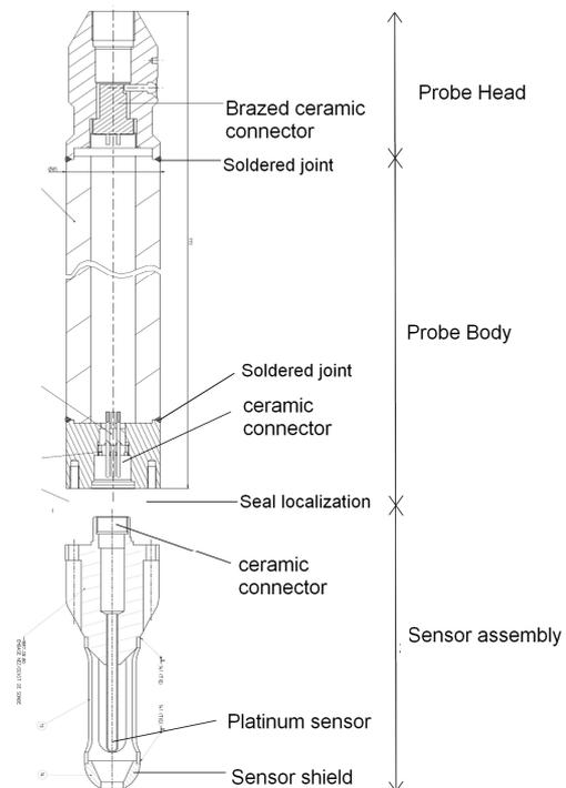
**Figure 2: Design of the BRGM wireline temperature sensor.**
