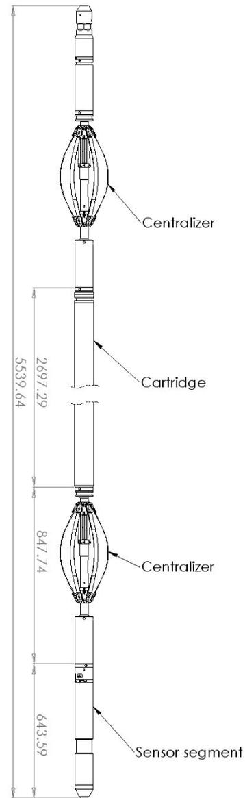
**Figure 5: Televiewer ABI92 with in-line centralizer**
