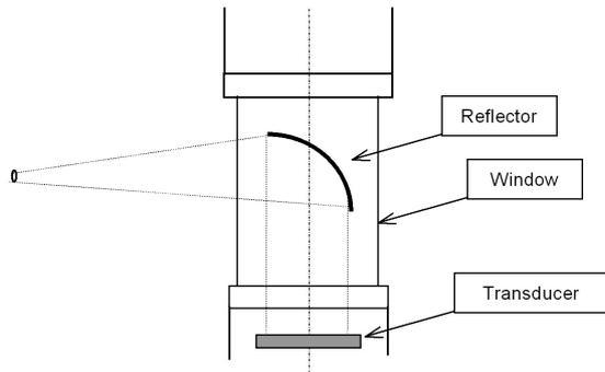
**Figure 4: Principle of the acoustic sensor.**
