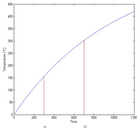
**Figure 1: A heat shielded instrument is placed in a 600°C environment. Over time, the internal section heats up from 0 degrees to the environment temperature. If the internals survive at 300 °C, the operational time is longer ( $t_2 > t_1$ ). Double temperature tolerance more than doubles the time duration.**
