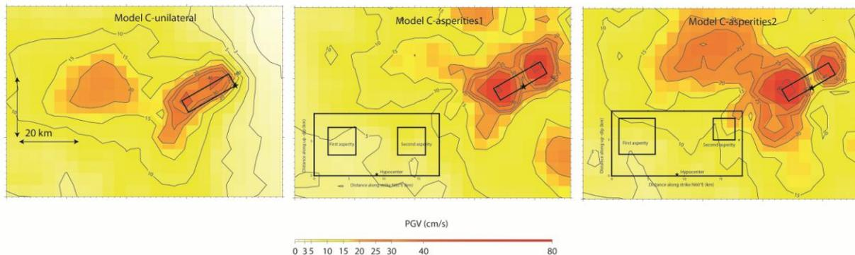
**Figure 5.** Horizontal PGV map for the derivative models based on fault geometry model C. ModelC-unilateral: Hypocenter is chosen eastern bottom corner of fault, and fault slip is uniform. ModelC-asperities1: Hypocenter is center bottom. Two asperities of equal dimension (10% each) are given. ModelC-asperities2: Hypocenter is center bottom. Two asperities of large (15%) and small areas (5%) are given.
