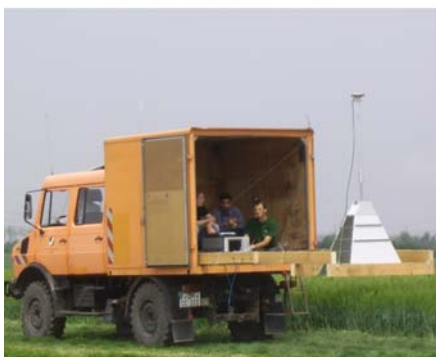
Fig.7.5 Real-time mapping of soil surface water content with advanced GPR (Lambot et al., 2006)
